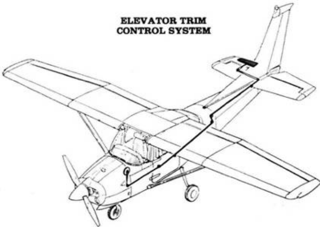
Figure 7-1. Flight Control and Trim Systems (Sheet 2 of 2)
