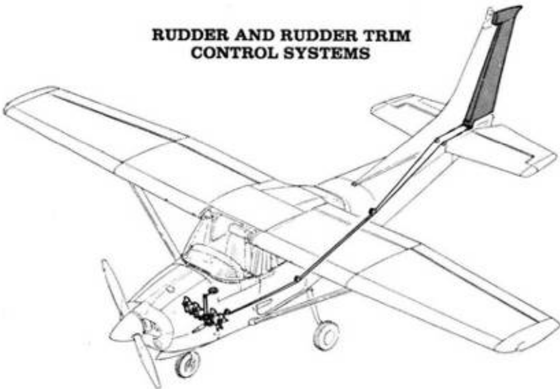
Figure 7-1. Flight Control and Trim Systems (Sheet 1 of 2)
